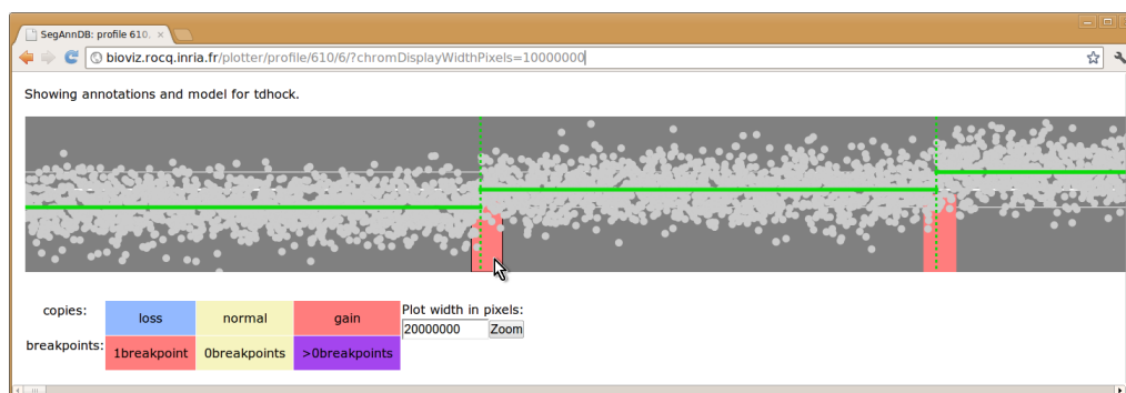
Figure 3.6: SegAnnDB chromosome detail page zoomed in. The signal in green is obtained from the grey data points using the \text{cghseg.k} model \hat{y}^k , with the number of segments k selected using the breakpoint annotations.
